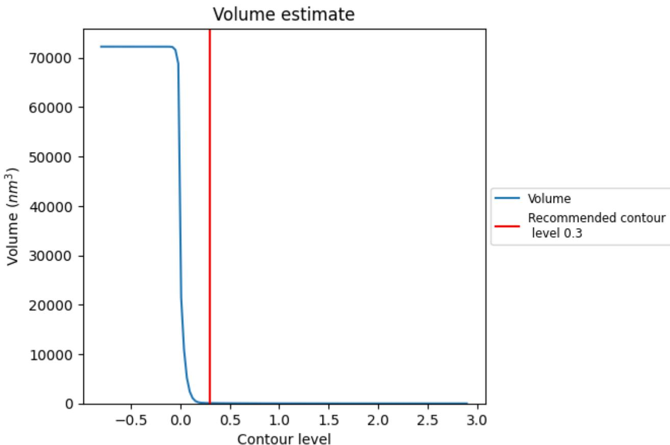
The volume at the recommended contour level is 72 nm<sup>3</sup>; this corresponds to an approximate mass of 65 kDa.
